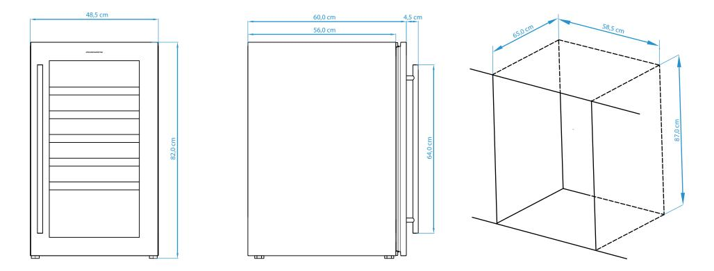
This model is designed for free-standing installation. Built-in installation is possible if the wine cooler has at least 5cm space on each side (like the above drawing). The air should be able to move freely in the space around the wine cooler.
